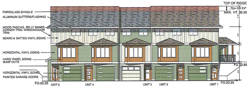
SIDE ELEVATION FROM DRIVEWAY (SIDE) scale 1/8"=1'-0"
